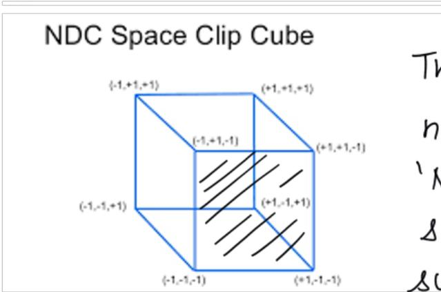
The projected point  $P(x_p, y_p, z_p)$  needs to be mapped to OpenGL's 'Normalized Device Coordinates'. (The shaded plane maps to your monitor screen.)
